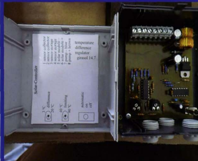
Temperature Differential Controller (TDC)
